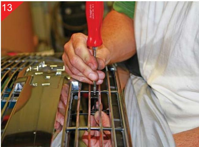
13 With grille face up place billet grille into the opening and center. Place supplied 2" bolt through mounting tab in billet grille, bracket goes on the backside and attach as shown. Snug down and contine with (3) remaining brackets.
