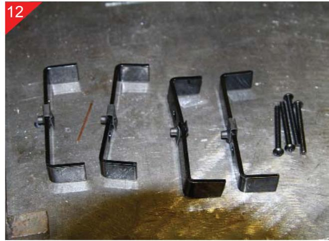
12 Next you will be installing for the top portion of teh billet grille. Locate the (4) upper brackets and attach supplied u-clips to center hole location in brackets as shown.
