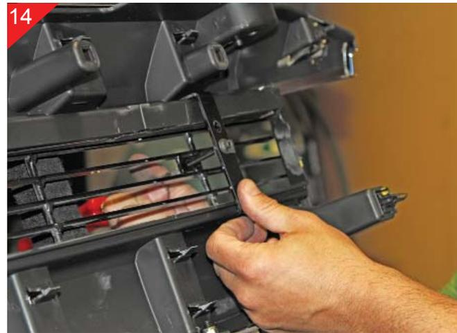
14 Continued with placement of the top brackets with brackets snug check alignment of the billet grille then fully tighten in place.
