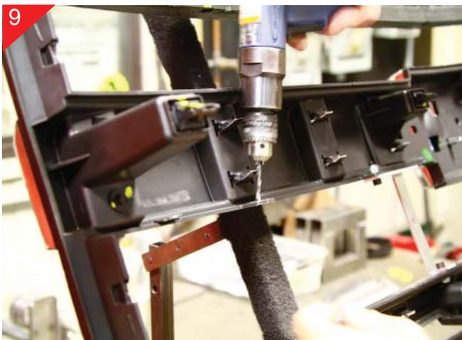
Next you will have a 2 step drilling process for each of the just marked center lines. Starting with  $\frac{1}{8}$ " drill bit then going to a  $\frac{1}{4}$ ".
