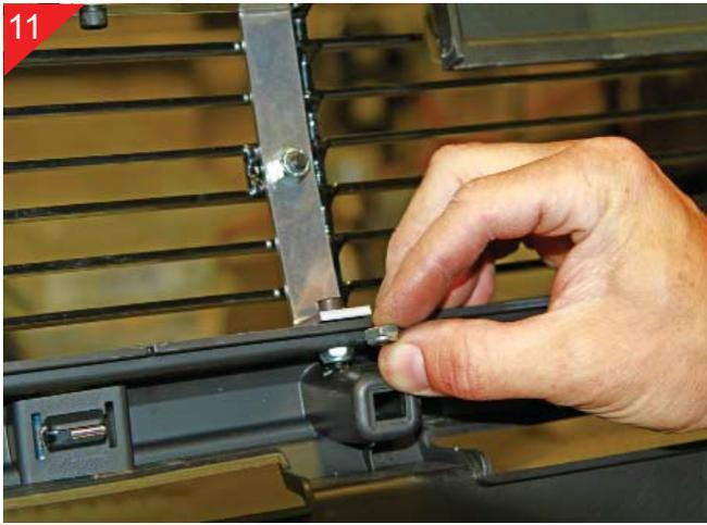
11 Install the bottom inner brackets. Same procedure as before except you will need to use 1/4-20 half nut nyloc nuts for securing in place..
