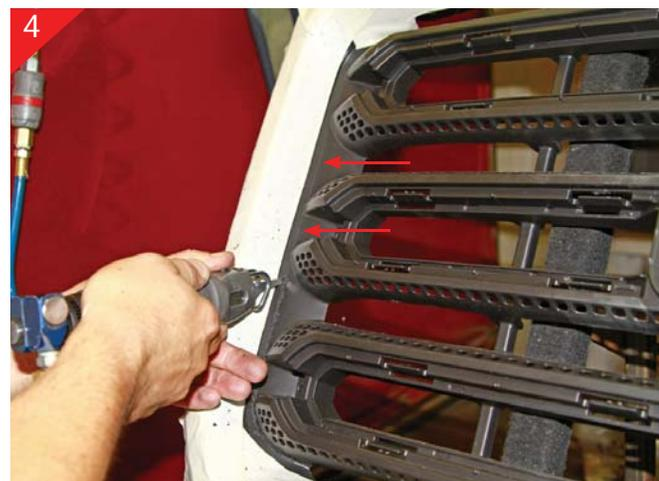
4 Continued cutting of the passenger side of the grille shell again following the line in the grille shell.
