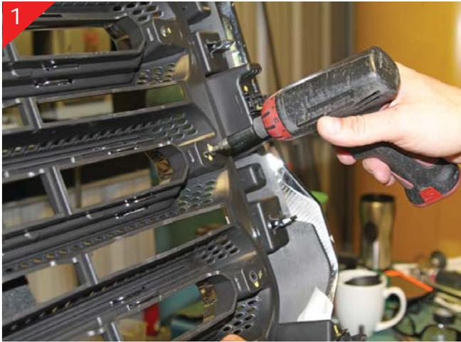
1 Remove stock shell and place on protective work surface. Next remove (6) screws from the backside holding chrome accents in place to the face of the stock grille shell.
