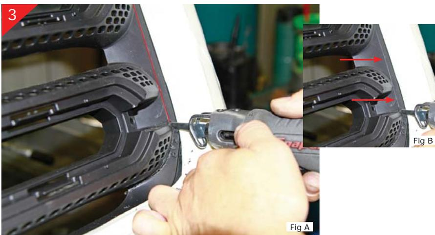
3 Next you will be cutting the center portion of the stock grille shell. Starting in the lower right hand corner follow around as shown above using an air saw or cut-off wheel. There is a molded line in the grille shell to follow shown above in RED. (Fig B shows actual line). You will cut both the driver and passenger side of the grille shell then move on to the top and bottom portion.
