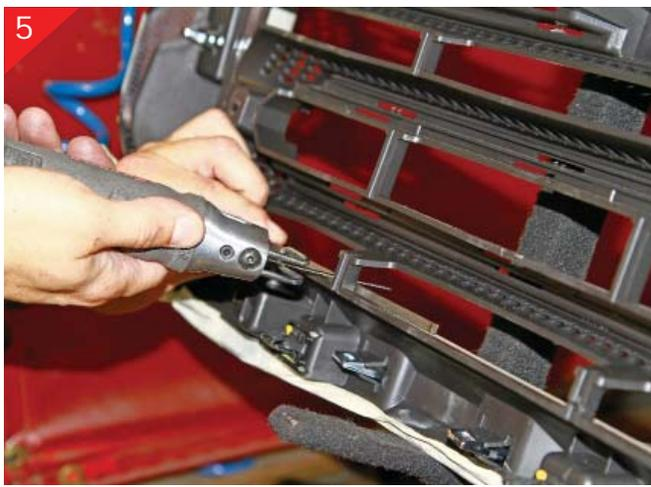
Next you will cut the bottom portion of the stock grille shell. We used a square piece of  $\frac{1}{4}$ " steel as a guide. You need to leave a  $\frac{1}{4}$ " of material to retain the bottom portion of the billet grille. Cut all the vertical attachment points along the bottom again using a guide to cut with making sure to leave material to retain billet grille.
