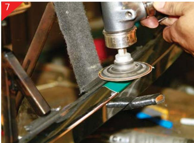
7 Using a sanding block or air sander, sand all the stand-off cut areas smooth just to clean up after cutting.
