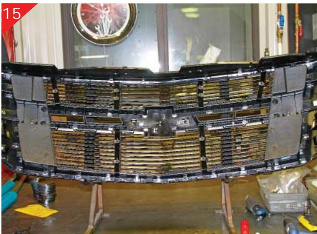
showing the backside of the grille shell with all brackets attached.
