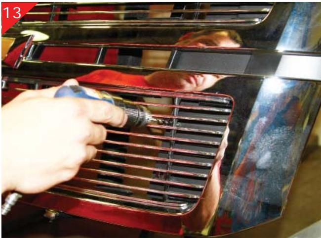
Using a 7/32" drill bit, drill thru the mounting tabs into the air dam that's located behind as shown above. Repeat for remaining side driver or passenger side.
