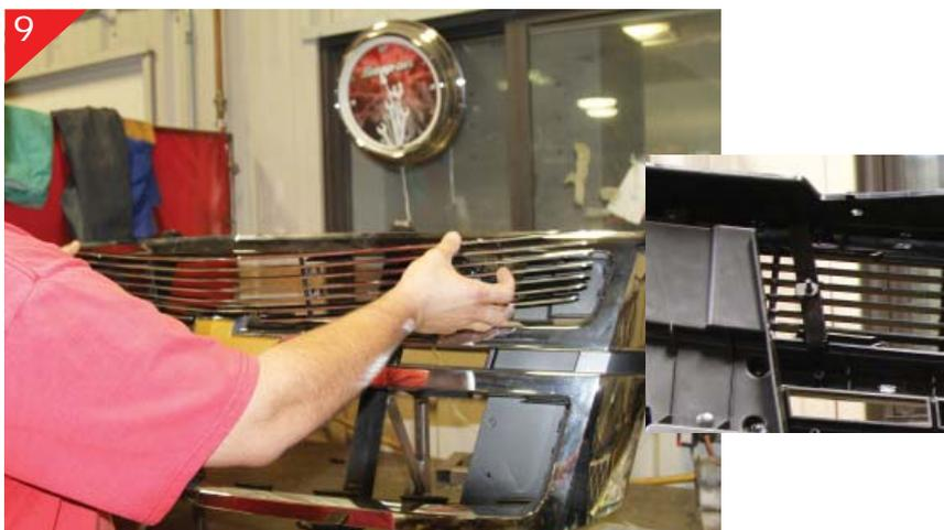
9 Turn bracket horizontal to place billet grille into opening and center. Rotate brackets around to catch the outer opening of the grille shell. Check to see that grille is centered then with the bracket match the angle of the air dams and tighten in place.
