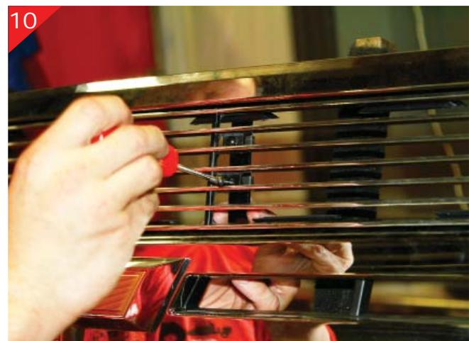
10 Place supplied clips on the (2) remaining upper center brackets and attach with the 10-24 x 1 1/2" bolts as shown.
