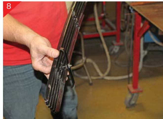
8 Starting with the upper portion of the billet grille. Attach outer bracket to billet grille as shown using the supplied brackets and 10-24 clips. Place clip on bracket attach bracket using 10-24 x 1 1/2" bolt.
