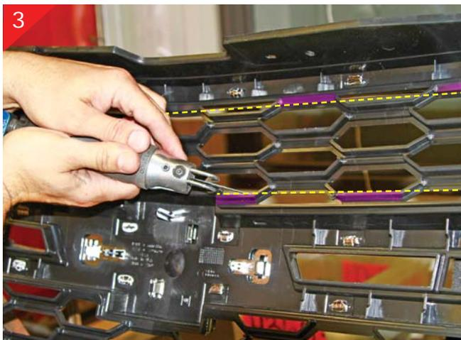
Next you will be removing the center portion of the stock grille shell. Do so by using a air saw or cut-off wheel to cut plastic shell. Make sure to leave the portions in purple DO NOT remove. This retain the billet grille into the opening. You will need to repeat the process for both the upper and lower portion of the grille. (See step 5 to help identify what needs to be left in place).
