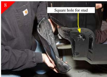
Place the corner piece on vehicle with the stud going thru the stock square hole. When placing corner piece let inner lip tuck around the support bracket. Attach corner using supplied 10-32 flange nut and washer.
