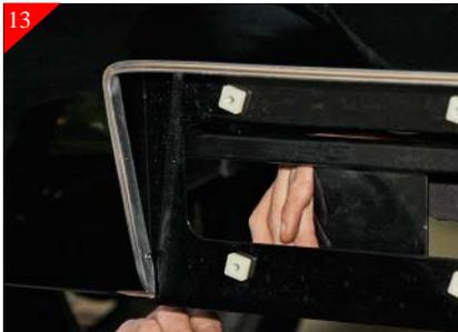
Locate the holes placed in the back side of the roll pan directly behind license frame area. Place the supplied 10-24 fender clips on these holes. Attach roll pan to the cross bar by using the supplied 10-24 x 5/8" bolts.
