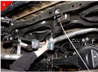
Attach using the supplied 5/16-18 x 3/4" bolt with the 5/16" washer on the top side and 5/16-18 nyloc nut to secure.
