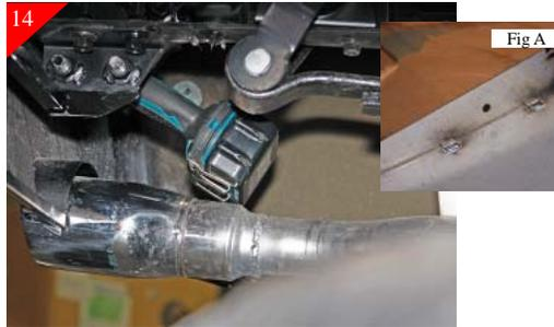
Locate the pre-drilled hole in each end of the roll pan shown in (fig A). Using the pre-drilled hole as a guide drill into plastic of the corner piece using a 1/4" drill bit. Secure each end of the roll pan using the supplied 1/4-20 x 3/4" and 1/4-20 nyloc nuts.
