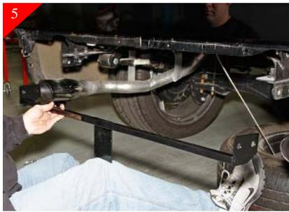
Locate the roll pan support cross bar.
