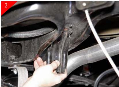
Locate and remove the (2) bolts holding the spare tire centering brackets. Do so by drilling the rivets holding the brackets in place using a 3/8" drill bit.
