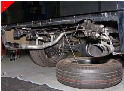
Start by completely dropping the spare tire. Do so by following the manufactures instructions for lowering the spare tire.
