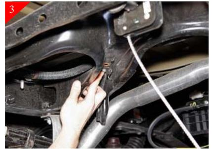
Next slide the bracket back by one hole as shown.
