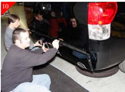
Use of a second person to help hold roll pan in place will be necessary. Place roll pan into opening and center.
