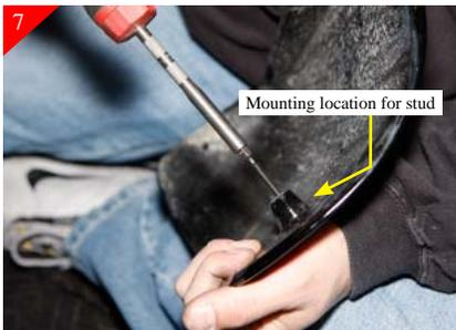
Locate the supplied corner pieces and attach the 10-32 x 1 1/4" stud in the mounting location shown above.
