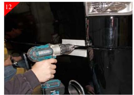
Locate the holes across top of roll pan, use these hole to attach roll pan. Tape using masking tape across the top of the roll pan and bottom of tail gate. This will protect both pieces during the attachment of the roll pan. Using the supplied self tapping screws attach roll pan as shown above. Note: when attaching roll pan place self tapping screw directly in the middle of the hole, this will give to a little adjustment for fine tuning the alignment.
