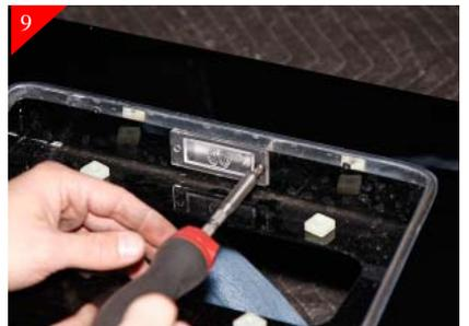
Install the license plate light by using the supplied 10-24 x 3/4" stainless steel bolts and 10-24 nyloc nuts without overtightening. Overtightening can cause the plastic light lens to crack.
