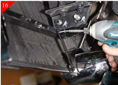
Attach straight bracket to bottom of the roll pan using the pre-drilled hole. First place supplied 10-24 fender clip on pre-drilled hole and attach bracket using 10-24 x 3/4". Then attach to the cross bar as shown using the supplied #8 x 3/4" self tapping screws.
